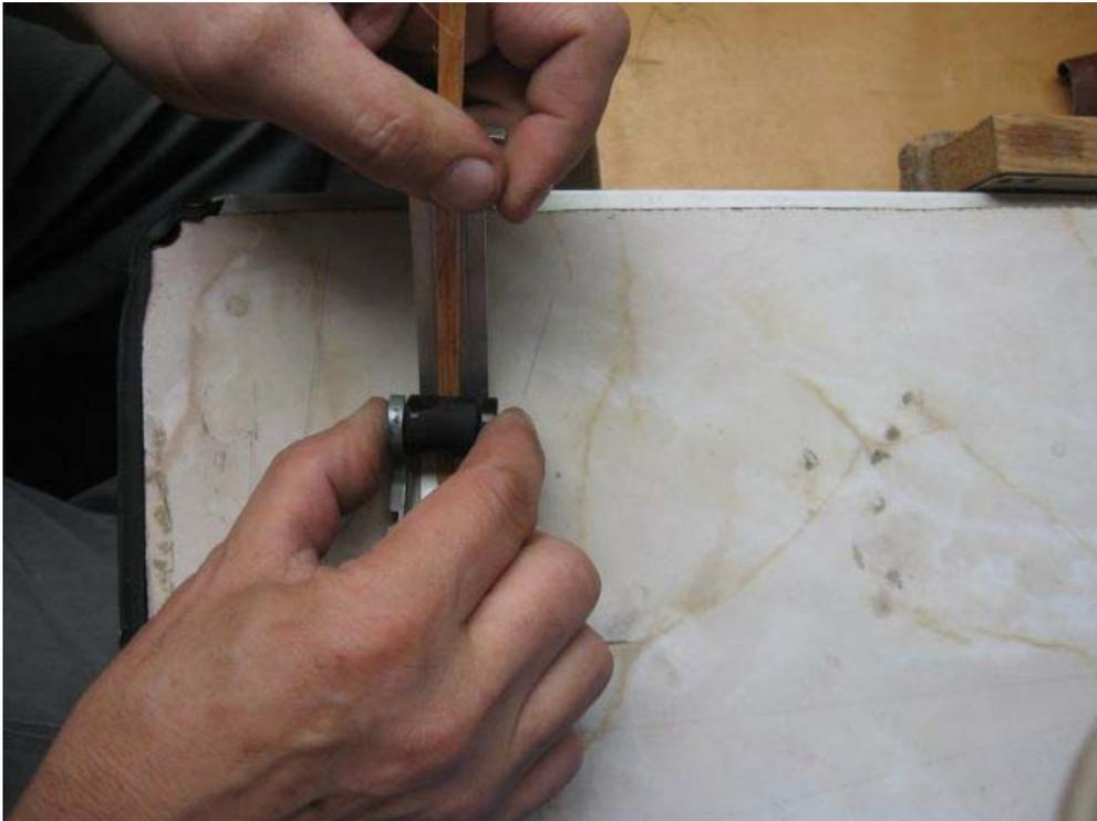
**Figure 12. – Using the Pinch Roller to Bend a Plank.**
