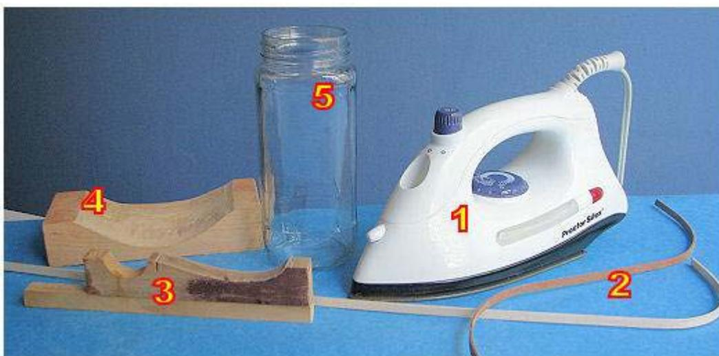
**Figure 1. – Plank Bending Jig and Tools.**
