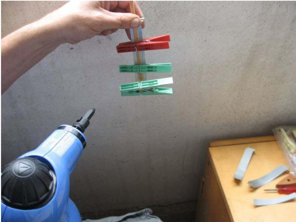
**Figure 14. – Steaming the Plank on the Jig.**
