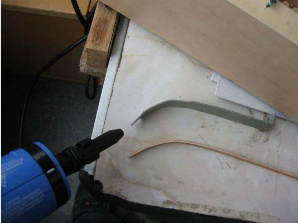
**Figure 5. – Planks Drying on the Shaped Metal.**
