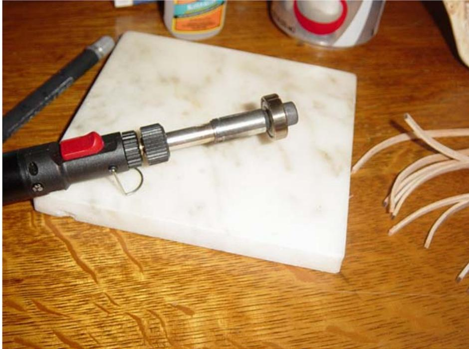
**Figure 1. – The Modified Bending Tool.**
