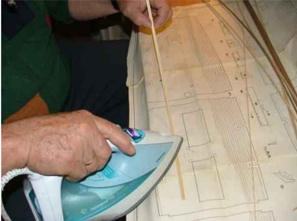
**Figure 1. – Applying the Steam iron to a Strip.**
