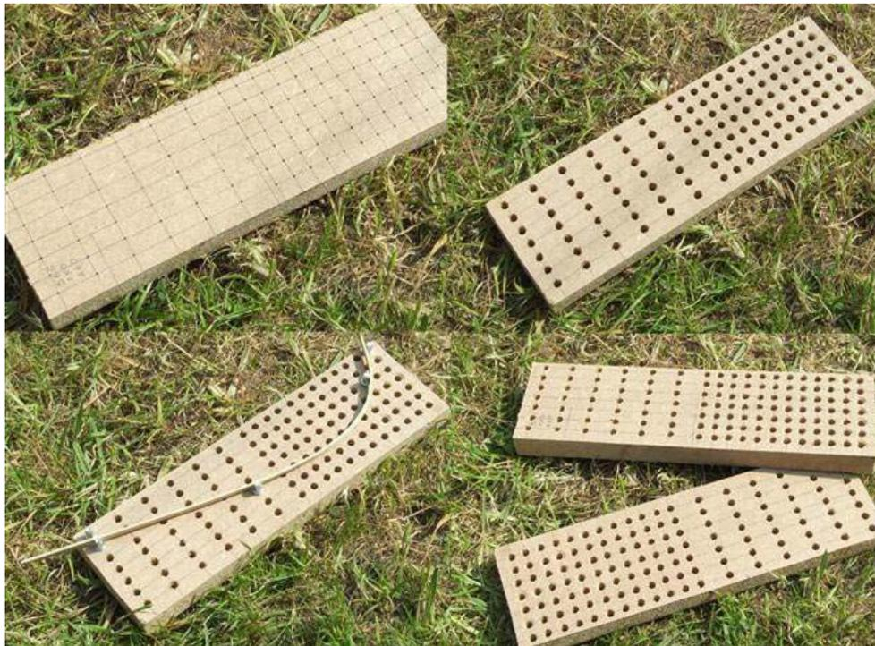
**Figure 1. – Plank Bending Jig.**
