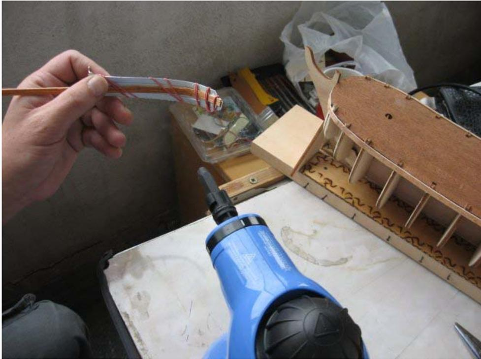
**Figure 3. – Applying Steam.**
