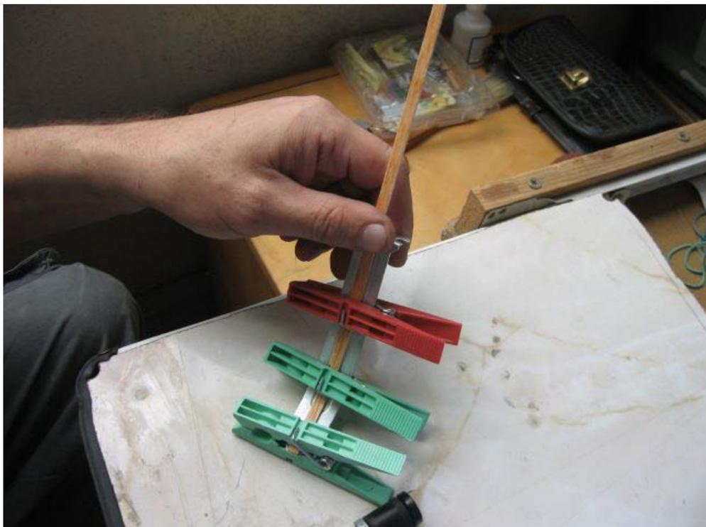
**Figure 13. – Clamping the Plank to the Jig.**
